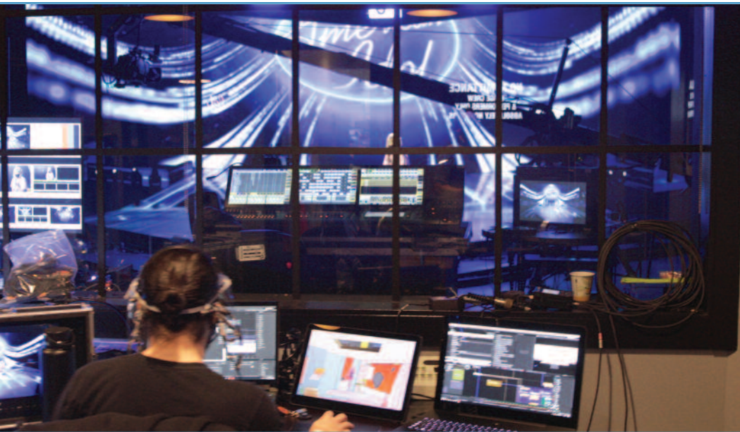
"In the control room," Hallaert says, "we have a Grass Valley Kayenne, audio is run through the Calrec Artemis [console], and for live performances we also run a DiGiCo SD10 console and a Yamaha CL5 Dante control mixer."
